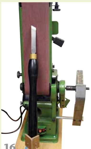
Here is the machine in action, sharpening a skew chisel. For easy repeatability, the sliding V block indexes against marks on the blue tape. I removed the rubber feet from the sander and used five #8 x 1/4" panhead screws to mount the sander on the wooden base.
