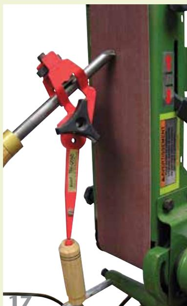
The Tru-Grind gouge-sharpening jig pivots in the socket turned into the top of the jig-holding sleeve.
